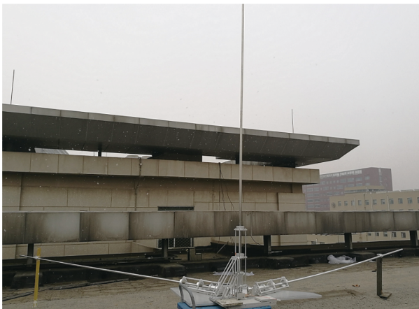
图10 低频射电频谱仪安装在楼顶进行空间电磁波接收试验的照片 Fig. 10 Photo of VLFRS installed on the rooftop to receive space electromagnetic waves
