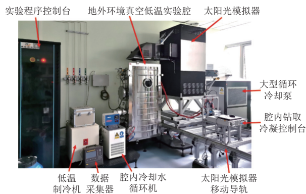
图6 低温真空环境模拟实验平台 Fig. 6 Image of integrated experimental system
