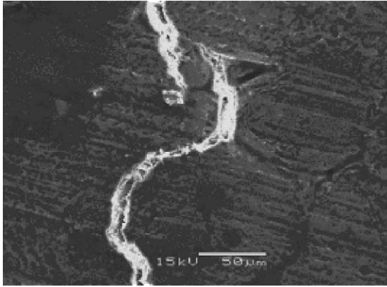
Fig. 6. Cracking along particle boundaries.
