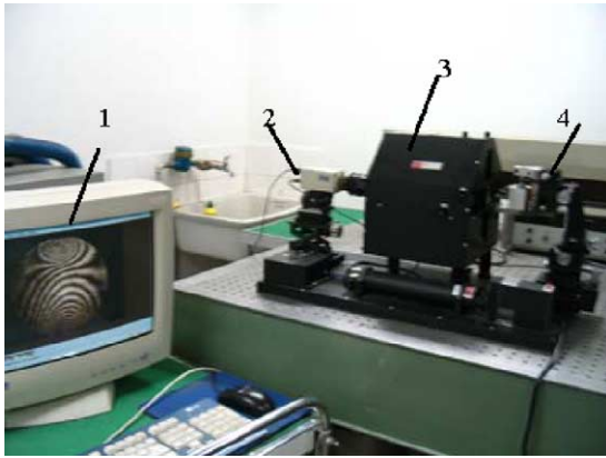
Fig. 3. Photography of the moiré interferometry system. 1, Computer; 2, CCD; 3, moiré interferometer; 4, the loading stage.
